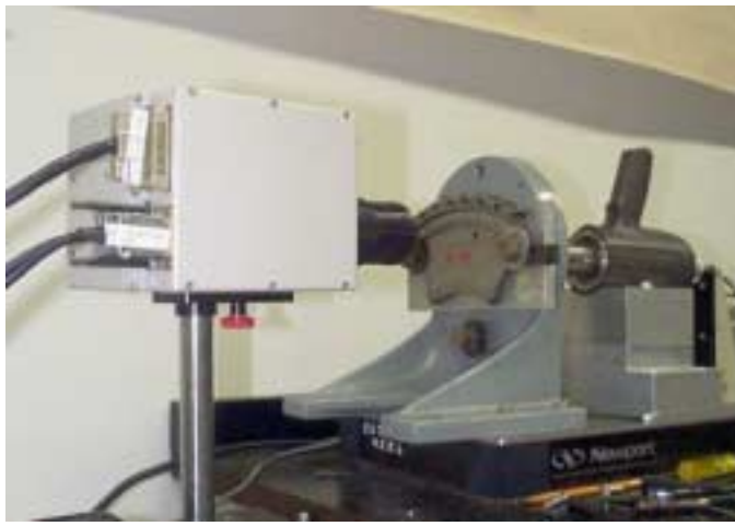
FIGURE 11 – Inspection of Compressor Disk using Sonic Thermography
