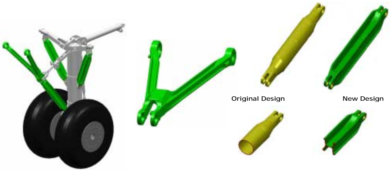
FIGURE 13 – Landing Gear Side Brace and Drag Strut Redesign
