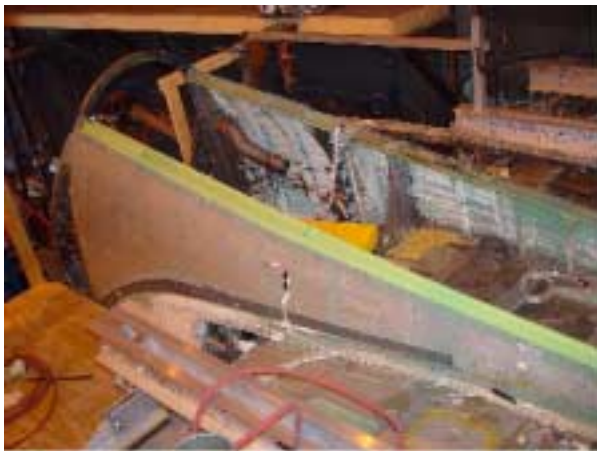
FIGURE 12 – One-piece Nacelle Upper Longerons
