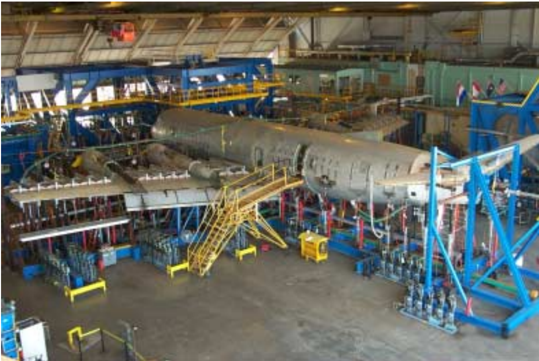
FIGURE 3 – P-3C Full Scale Fatigue Test Article
