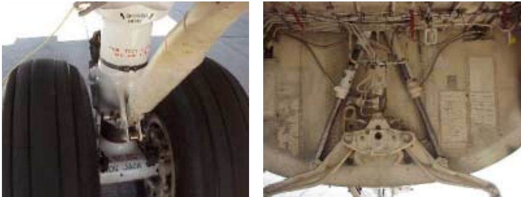
FIGURE 8 – HVOF Application on the P-3 Main Landing Gear Cylinder and Bomb Bay Actuators
