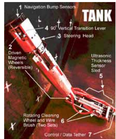
Fury remote-monitoring system for tank inspection.
