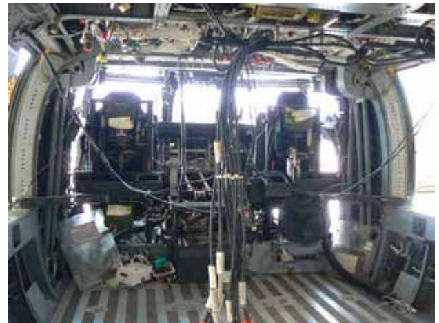
During a Reset overhaul, mechanics inspect and repair every inch of the Army Black Hawk, using corrosion prevention materials to protect the antennae, skin, and the floorboard interface. Photo by Cynthia Greenwood, CorrDefense.
