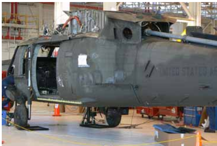
Built for European operations during the cold war, the Army's 60s-era Black Hawk was not designed to withstand the desert's salt, sand, and grit. Photo by Cynthia Greenwood, CorrDefense.
