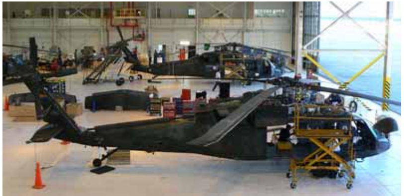
Under the Reset program, Army-sponsored mechanics refurbish Black Hawk helicopters returning from combat in Iraq and Afghanistan. Photo by Cynthia Greenwood, CorrDefense.
