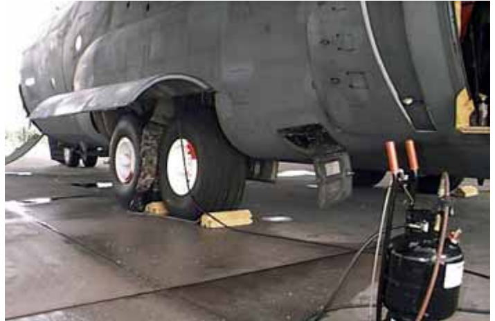
The Patrick AFB maintenance crew uses a fogging applicator to apply corrosion prevention compounds inside a C-130 wheel well. Photo courtesy of Patrick AFB.
