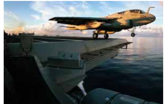
The Navy's EA-6B Prowler, a fixed-wing fighter aircraft, supports air strikes and ground troops by interrupting enemy electronic activity. Photo Courtesy of U.S. Navy.
