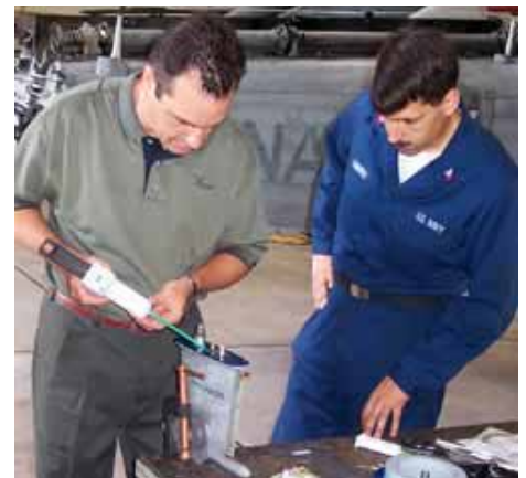
Dave Schmidt, Military Programs Manager at AvDEC, (left) works with Navy engineer Joshua Honaker to install antenna gaskets on an SH-60B aircraft, which was flown by the HSL45 Wolfpack squadron at North Island Naval Air Station during the Iraq war, in the summer of 2003.
