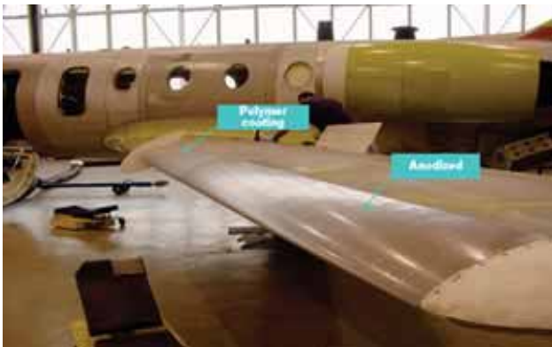
The color of a polymer coating used to protect the slat of a twin-engine Falcon resembles that of its anodized surface. Photo courtesy of U.S. Coast Guard.
