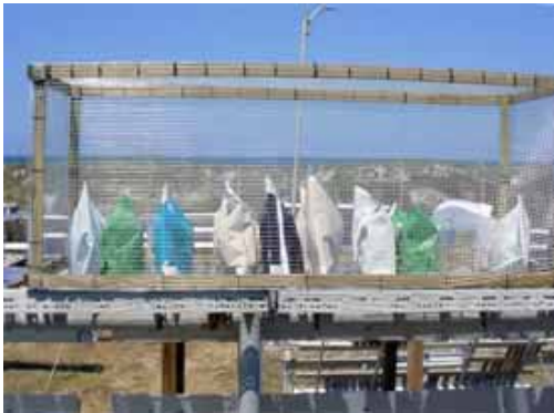
Materials engineers cover bagged test samples with a bird-proof cage to avoid tampering by wildlife. Photo courtesy of Air Force Corrosion Office.
