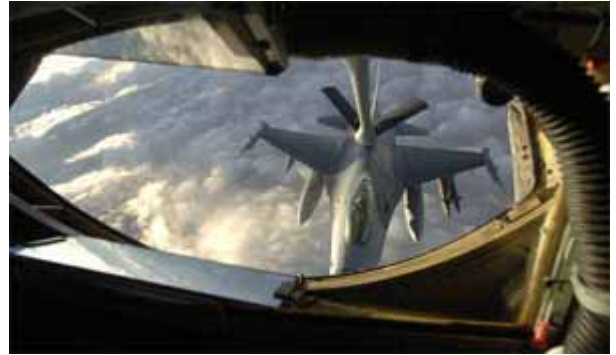
A KC-135 Stratotanker connects with an F-16 Fighting Falcon over Iraq to offload more than 20,000 pounds of fuel on October 23, 2006. The F-16 then resumed its close-air-support mission. Photo by M.Sgt. Scott Wagers, U.S. Air Force.
