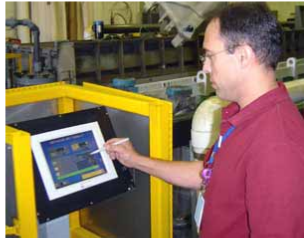
At the surface-finishing shop, Ruben Prado, a NADEP process control chemist, enters a "strategy" into the Metalast Integrated Process Controller (JobPro) before anodizing the main landing gear of a Navy EA-6B Prowler.
