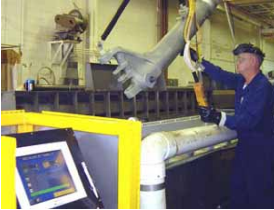
The main landing gear of an EA-6B Prowler is processed in a modified anodizing tank.
