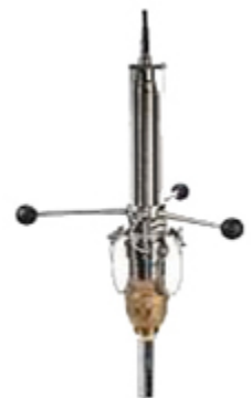
Researchers are testing commercially available sensors in Fort Bragg's water distribution systems to find and correct corrosion problems.
