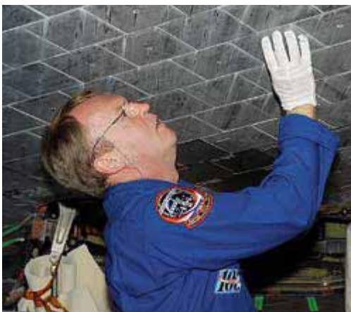
Mission Specialist Andy Thomas inspects thermal protection tiles on the Space Shuttle in 2005. Photo courtesy of NASA.
