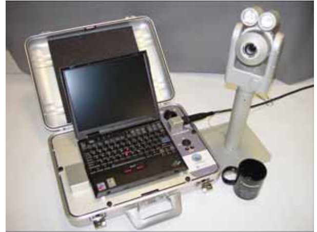
The Naval Research Laboratory is using an Insertable Stalk Imaging System (ISIS) to visually and quantitatively assess the condition of the coating inside a ship's ballast tank. Photo courtesy of Naval Research Lab.
