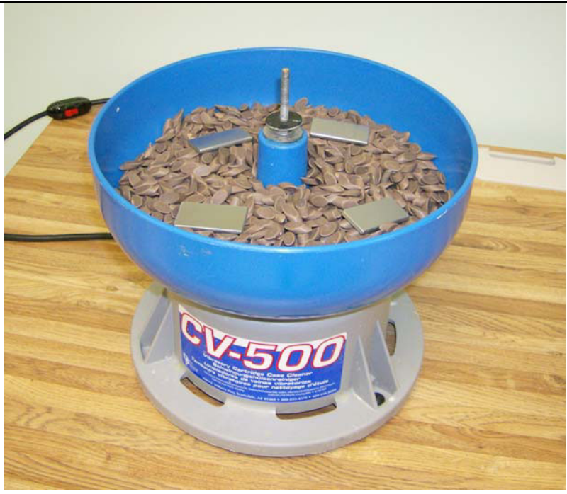
Figure 3: Small vibratory bowl with 11 inches (0.28 m) inner diameter filled with 4 kg of large ceramic media.
