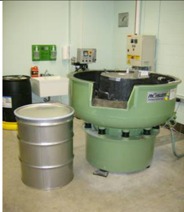
Figure 1: Big vibratory bowl with 45.5 inches (1.16 m) inner diameter and a dosing station in the background for continuous flow of chemicals through the bowl.
