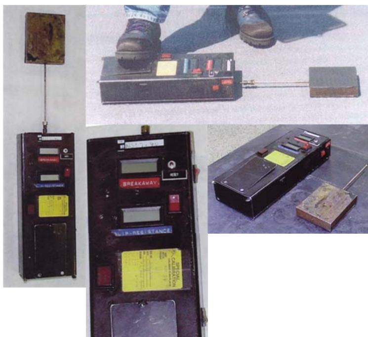
Figure 4: Portable NAVSSES Slipmeter design circa 1996
