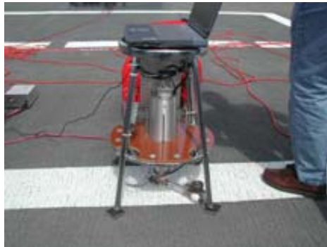
Figure 5: Early prototype of the portable ball-on-flat COF measuring device.
