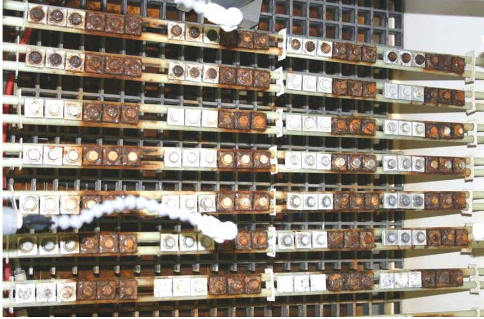
Fig. 1: Top view of the fastener assemblies inside the atmospheric exposure chamber.
