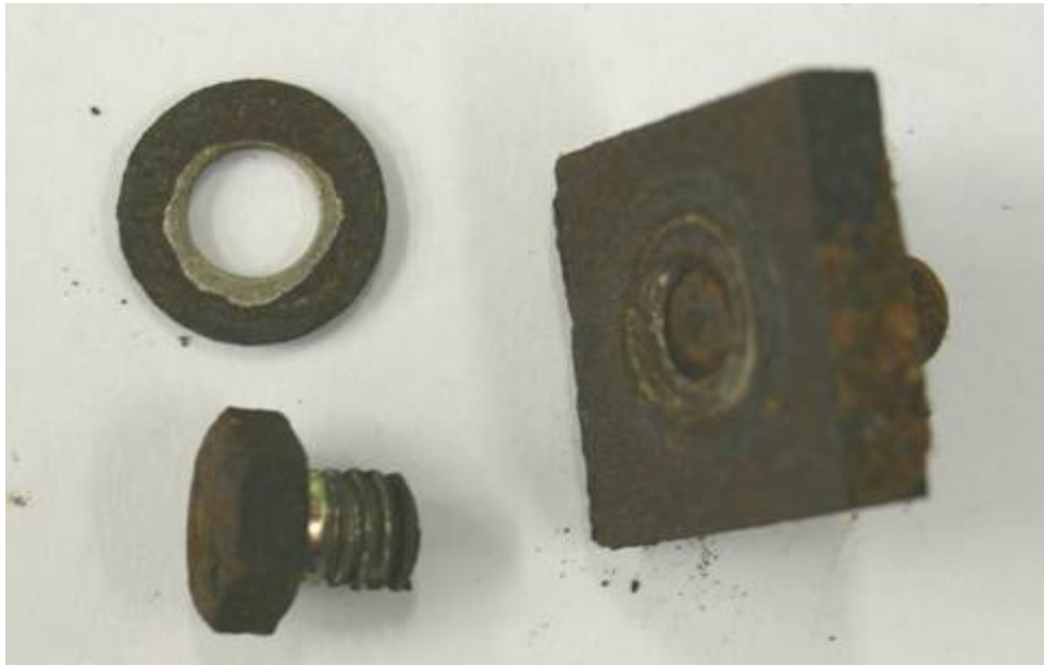
Fig. 12: Photograph of a broken untreated black oxide-coated bolt in a 1018 steel panel after 28 days of exposure. Severe galling/seizing was noted after 28 days of exposure.
