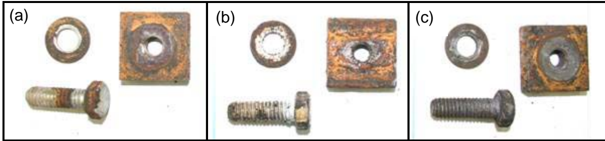
Fig. 13: Photograph of disassembled test pieces of cadmium-plated steel/steel panel assemblies after exposure in the atmospheric chamber for a period of 7 days. For the untreated fastener (a), thread corrosion is visible. The PTFE-treated bolt (b) still retained much of the white colored fastener treatment and the silver colored petroleum-based anti-seize (c) is also visible after 7 days.
